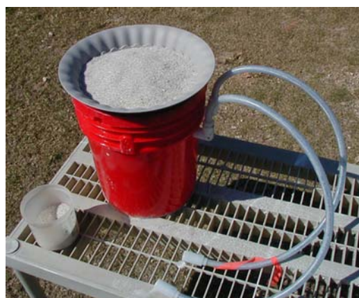
Figure 3. Lysimeter with sand placed in collecting plate and flexible tubing attached for sample collection Credits: Harry Trafford (c) UF/IFAS 2006
