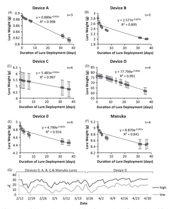
**Figure 5** Release rates of six *Raffaelea* odour dispensers and manuka oil lures. Release rates of device 0 (E), device A (A), device B (B), device C (C), device D (D) and manuka (F) are reported (mg/day). Each data set was fitted with an exponential decay curve; equation and  $R^2$  is shown for each device. Temperature highs and lows during gravimetric analysis of the lures are shown in (G).
